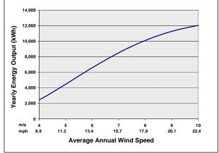
\*This distribution is based on the Power Curve data and the average annual wind speed (weibull distribution)
